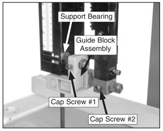
Figure 25. Back of upper blade guide.
